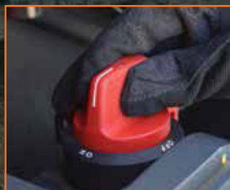
Battery cut-off switch
