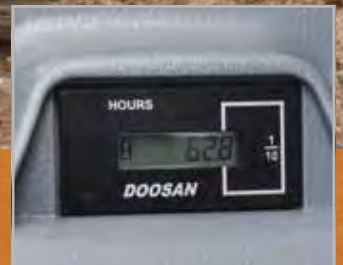
Hour meter (from ground level)
