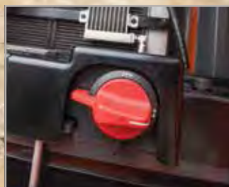
Battery cut-off switch
