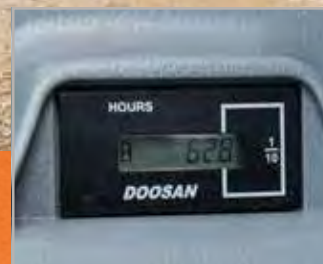
Hour meter (from ground level)
